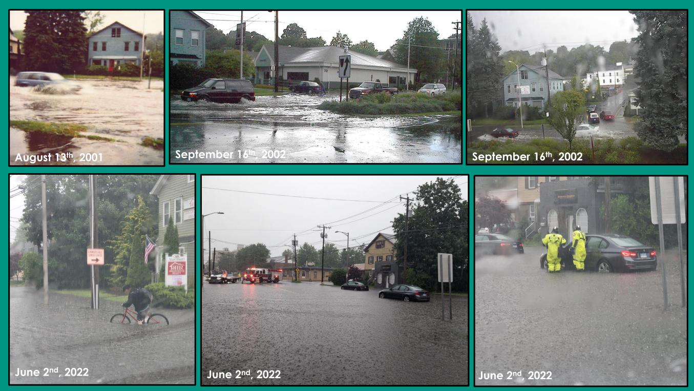
There is significant drainage-related flooding in Downtown Danbury as shown in the photos above, which were all taken at the Main Street and Elmwood Place intersection. Flooding occurs in the streets and, under certain conditions, extends onto adjacent properties and into basements.
