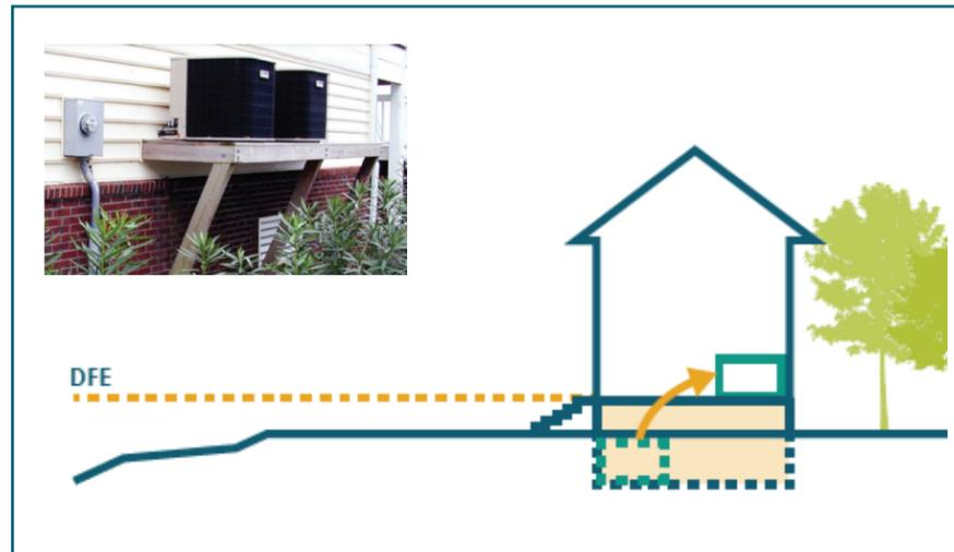
Relocating critical systems to higher floors within structures reduces the impacts of flooding on critical services and reduces recovery times. This tool increases the resilience of essential services to homes and businesses.
