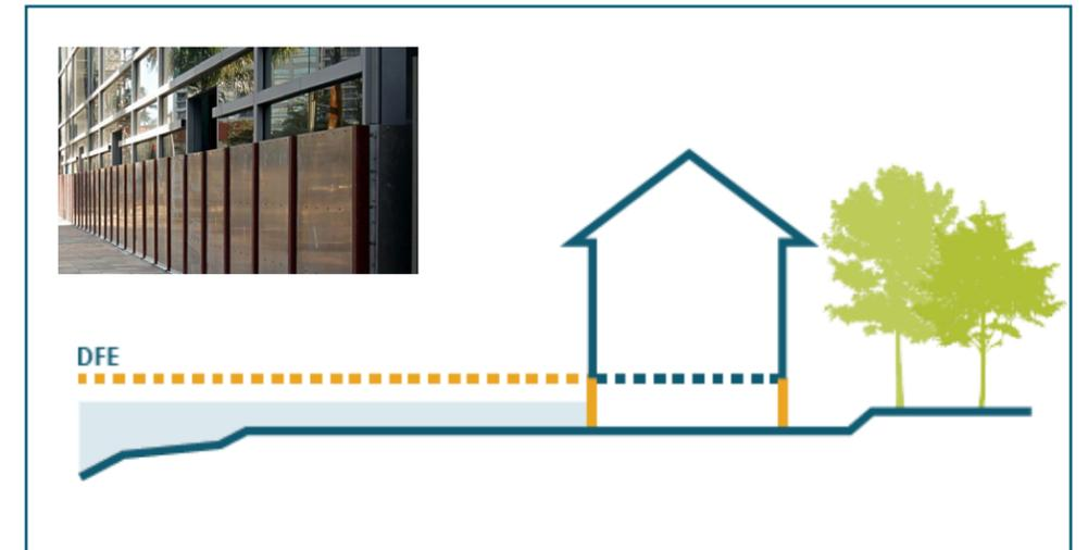
Wetproofing involves sealing susceptible levels to water infiltration. This allows for flood water to move into and through these levels while limiting infiltration to the rest of the structure. Dryproofing involves fully blocking out floodwaters with both permanent and deployable structures.
