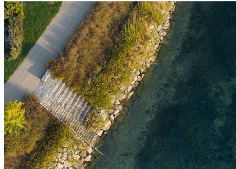
Revetments are hard sloping structures, typically constructed using natural stone, or concrete blocks designed to reduce shoreline erosion by absorbing wave energy and minimizing wave run-up. Sometimes these structured systems are necessary and can be altered as hybrid systems to incorporate ecological features providing enhanced habitat opportunities as well as enhance quality of life and water quality.
