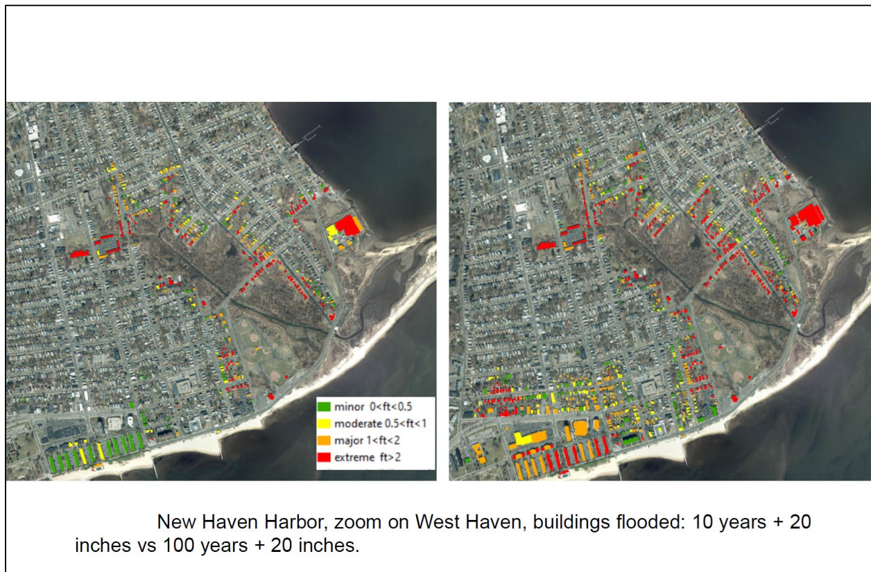
Caption: Evaluation of the extent of flooded structures and buildings under a scenario that includes elevation of Beach Street and First Avenue in West Haven, CT.
