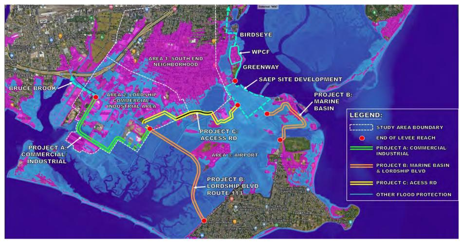
Figure 3: 2D Hydrodynamic Overland Flood Model – Comparison of inundation limits during Sandy 2012 (blue shading) and a 100-yr flood condition (blue + pink shading) with flood protection segments overlaid.
