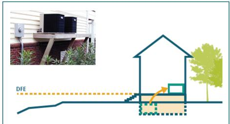
Relocating critical systems to higher floors within structures reduces the impacts of flooding on critical services and reduces recovery times. This tool increases the resilience of essential services to homes and businesses.
