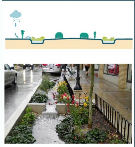
Right-of-way bioswales are vegetated drainage courses located in sidewalks to capture, detain, and infiltrate runoff from streets, allowing any excess rainwater to enter the piped stormwater system.
