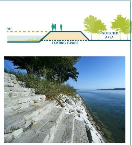
Berms are earthen mounds of various widths that provide flood protection and, where possible, public access to and along the waterfront. Where there is less space, berms can be narrow with a path on their crests. Where there is more space, they can widen to become elevated waterfront parks, creating places for communities to gather while simultaneously providing flood protection.
