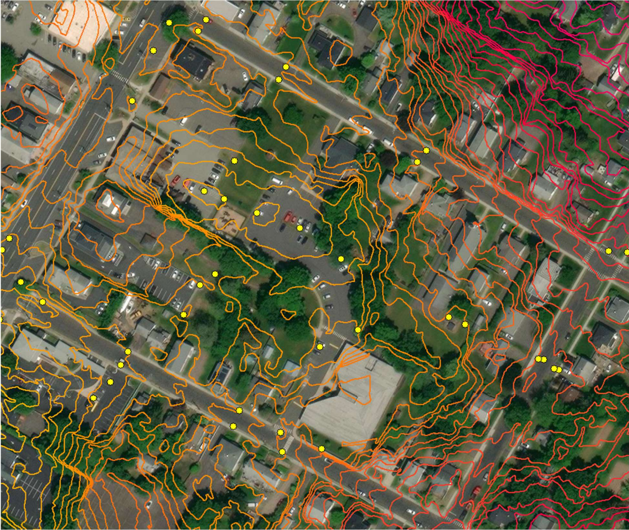
Figure 1: Contour data derived from 2016 LiDAR (red/orange lines) and spatially referenced catch basins (yellow dots) shown over aerial imagery for the Town of Portland.
