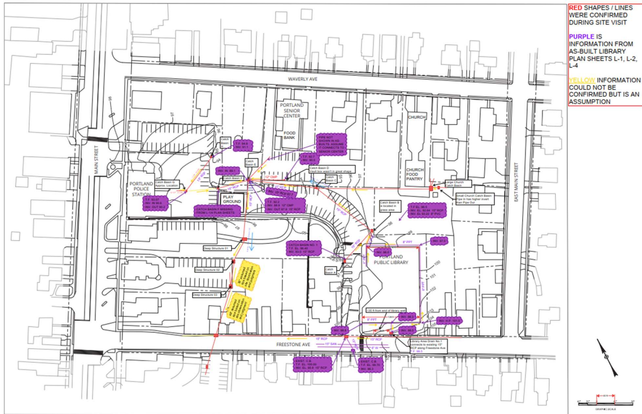
Figure 3: Representation of drainage network assembled from field notes.
