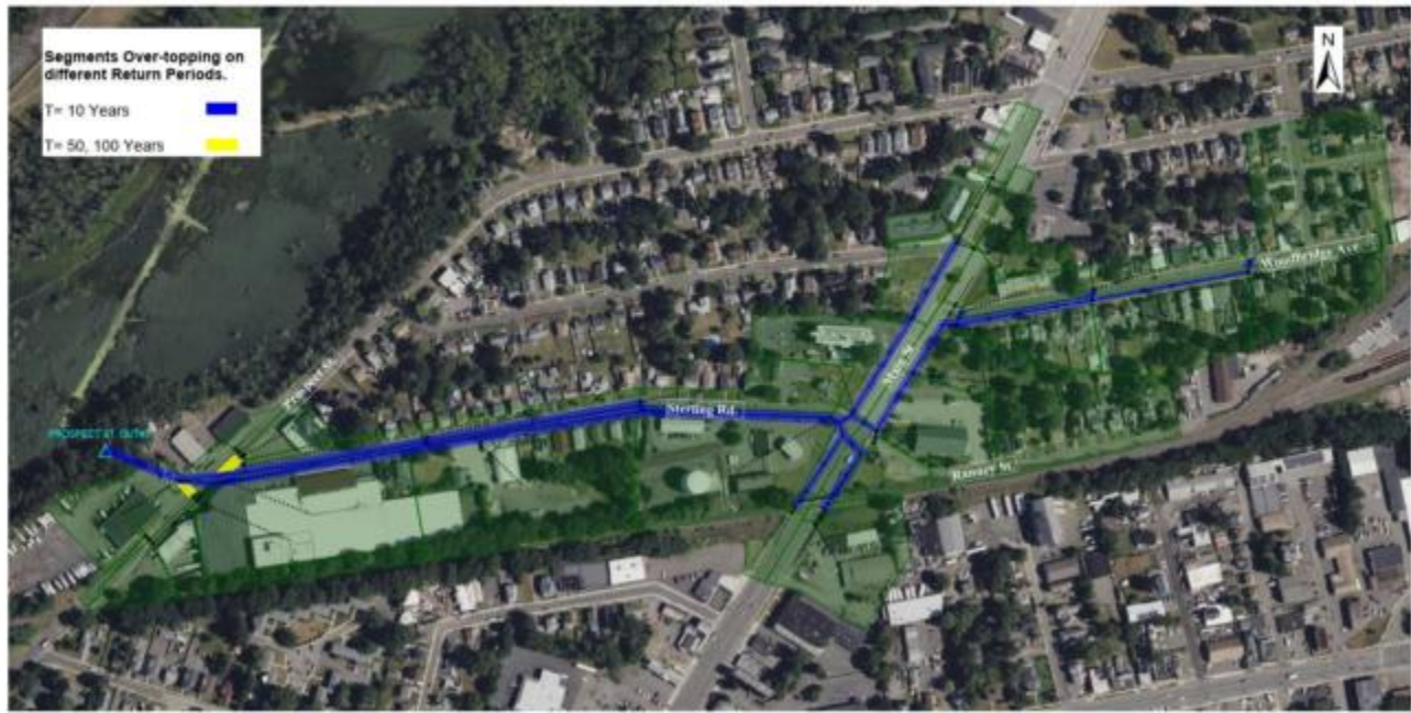
Figure 17. Future Conditions (2040-2069) - Over-topping During Various Storm Events
