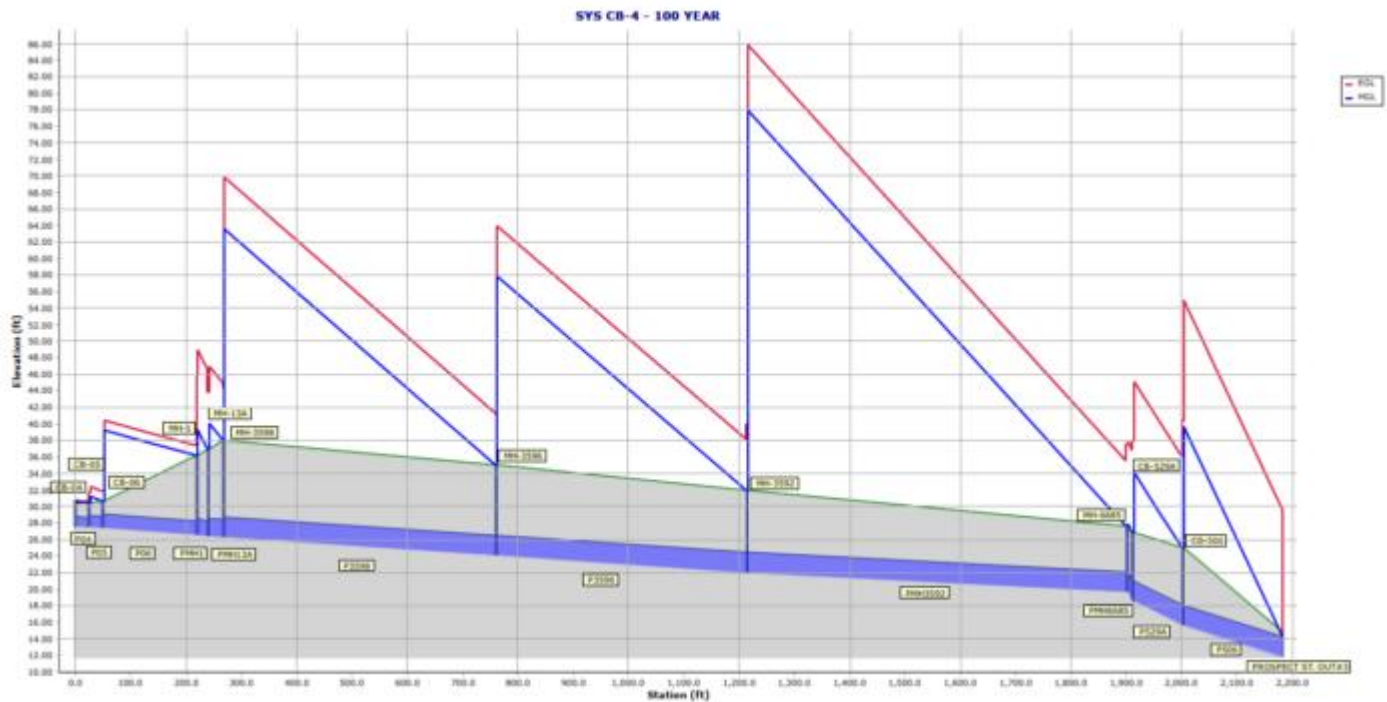
Figure 14. Existing Conditions - 100-year Pipe Profile
