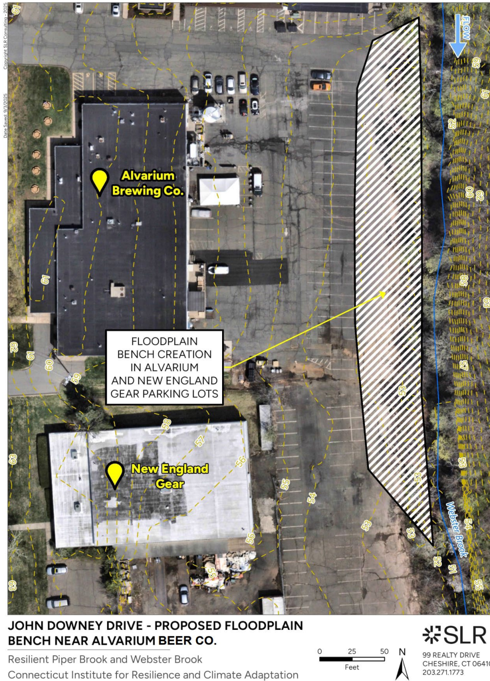
Figure 18: Concept Design: Alvarium Beer Company floodplain bench
