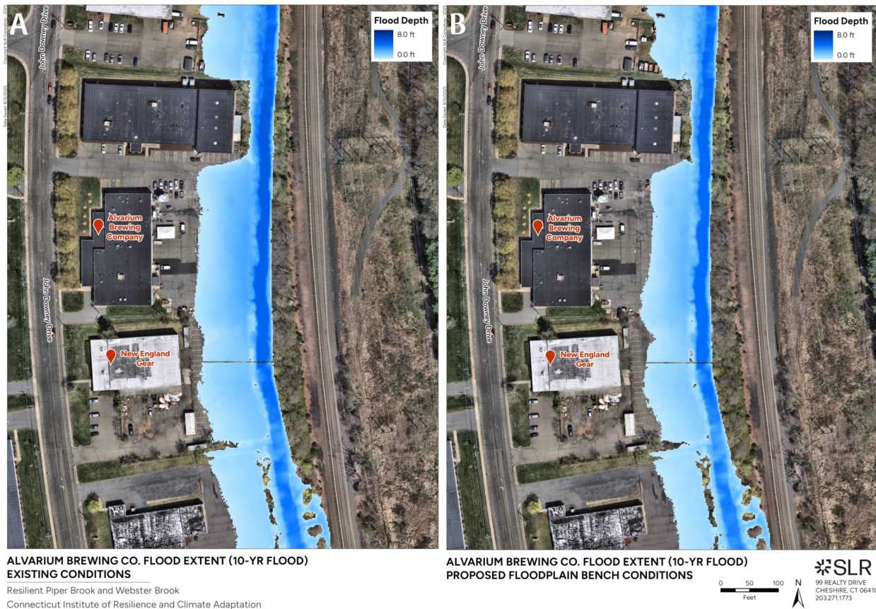
Figure 20: Water depth for 10-year flood for A) existing conditions and B) proposed measures
